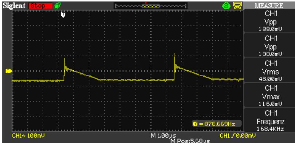
Because some (though inaudibly small) residues of the switching could be found too at the plate of the first triode when idling, I needed to reduce the ripple at the output. So the next step was to build an additional filter. I decided to use a small piece of FR4 (raw PCB material) to place the rectifier, the module and the additional output filter on it. You can see the finished part from this picture ->
