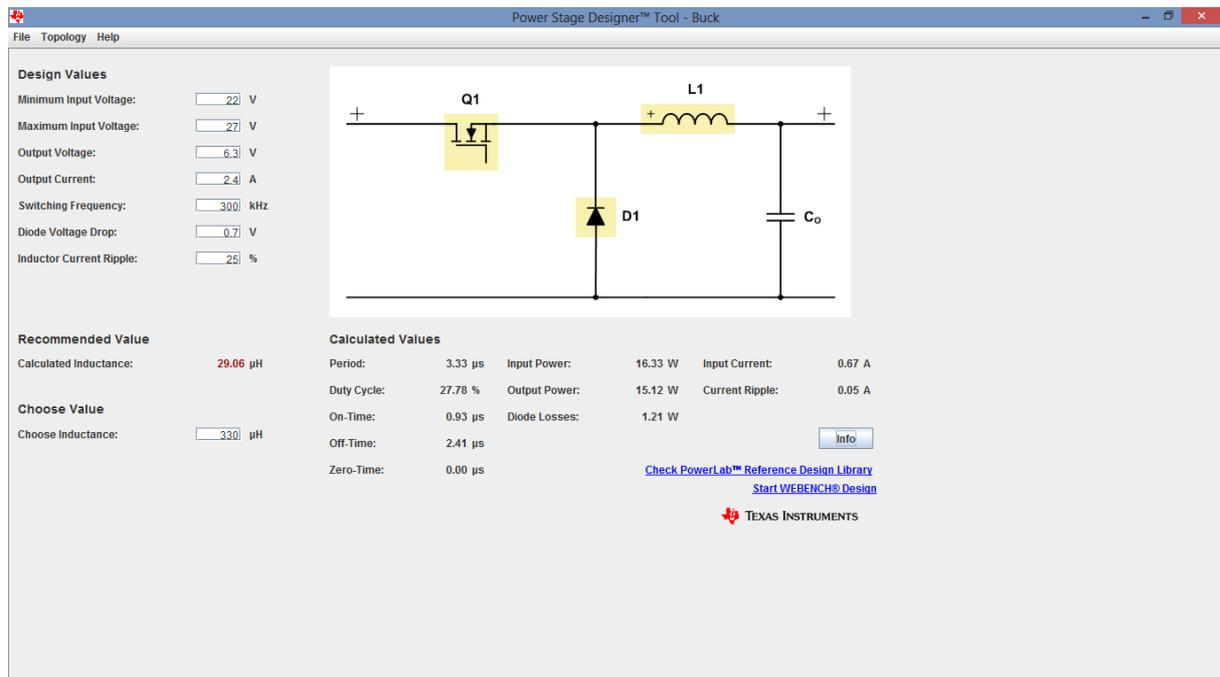
The difference between input- and output-power is shown as 1,2W. They are the losses of the diode only. In the real world, there will be losses from the switching transistor and the  $R_{dc}$  of the choke too. But over the thumb the efficiency should be in the range of 90%.
