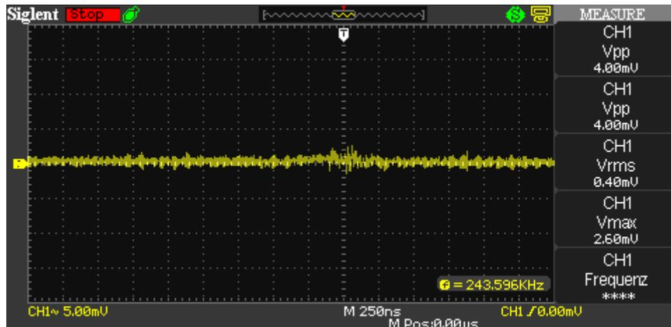
The situation is 6,3VDC, residual ripple is 0,4mVrms @ 300kHz and load current is 2,46ADC. Current limit was set to 2,6ADC.
