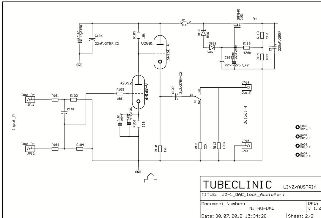
This time I used two power MOSFETS to decouple both tube-supplies and keep them free of noise. Again, I used a gyrator circuit. Q1 and Q101 form a choke "built of sand". This will keep the impedance of the supply chain to very low values while smoothing out the last ripple. The used MOSFET was chosen for its low  $R_{DS}$  and because it will withstand spikes from the supply line up to 500V. The voltage drop over the MOSFET will be app. 10VDC.
